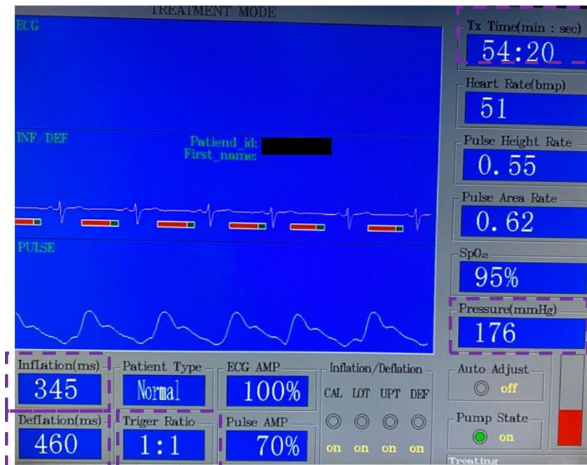
Fig. 7. Example of an ECP system display. The purple dash boxes are parameters that may be adjusted during the ECP treatment
