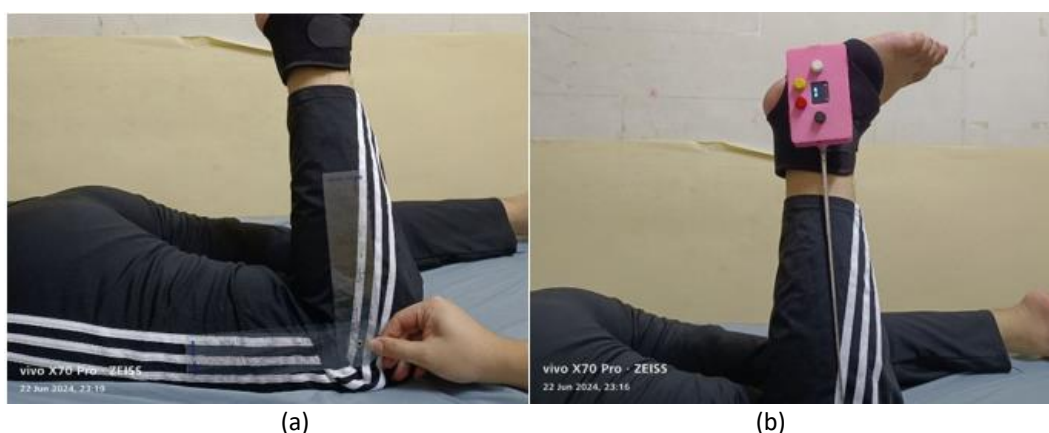
Fig. 10. Determination of AOP using (a) Goniometer (b) Angle Assist, A 2 prototype
