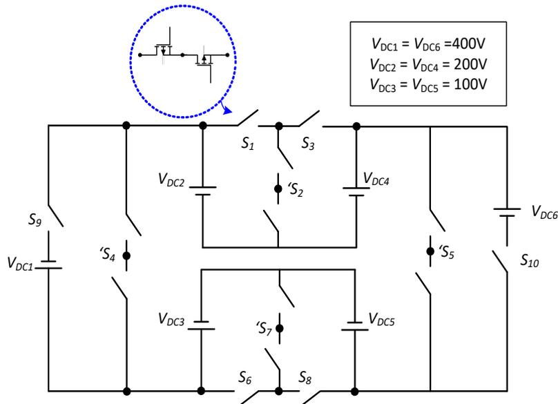
**Fig. 2.** Schematic of Topology II as adapted from [13]
