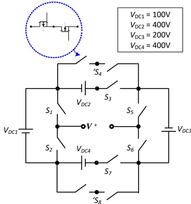
Fig. 1. Schematic of Topology I as adapted from [4]
