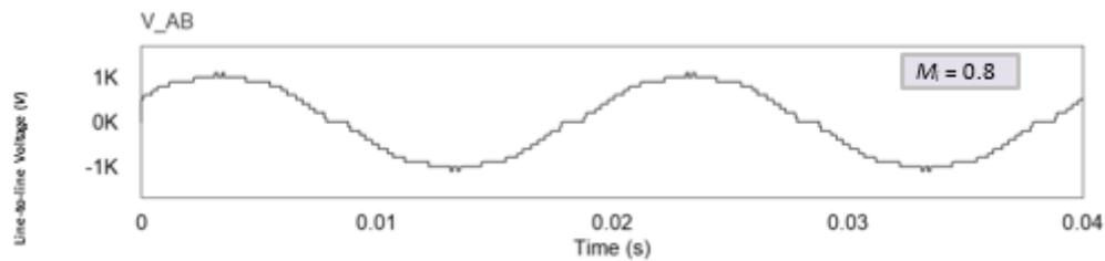
Fig. 5. Line-to-line output voltage of three-phase multilevel inverter
